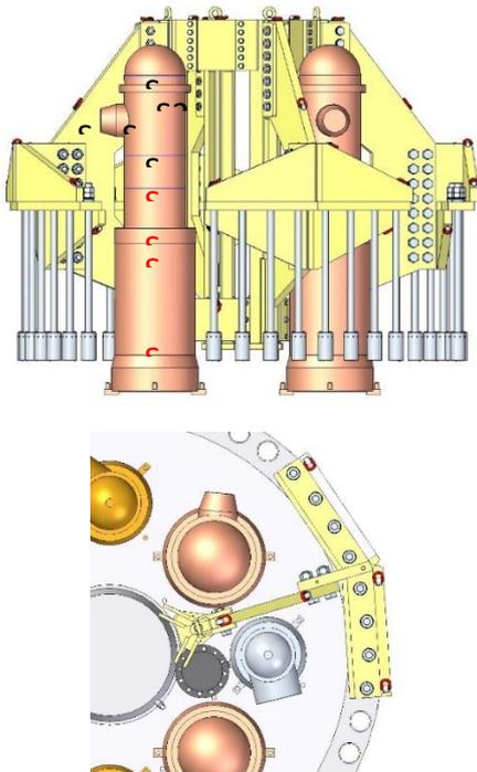
Figure 2 Elevation and plan of ESR in pod showing positions of superheater welds
