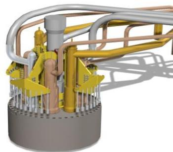
Figure 1 Illustration of ESR in BCU showing headers and tailpipes
