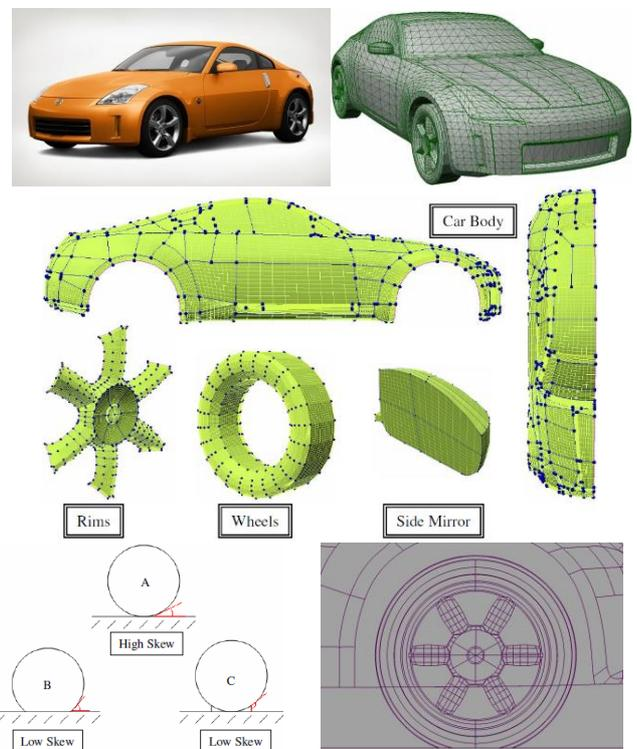
This reverse engineering method is particularly useful for design modification where fluid flow properties of the existing design can be replicated and compared against different operating scenarios.
